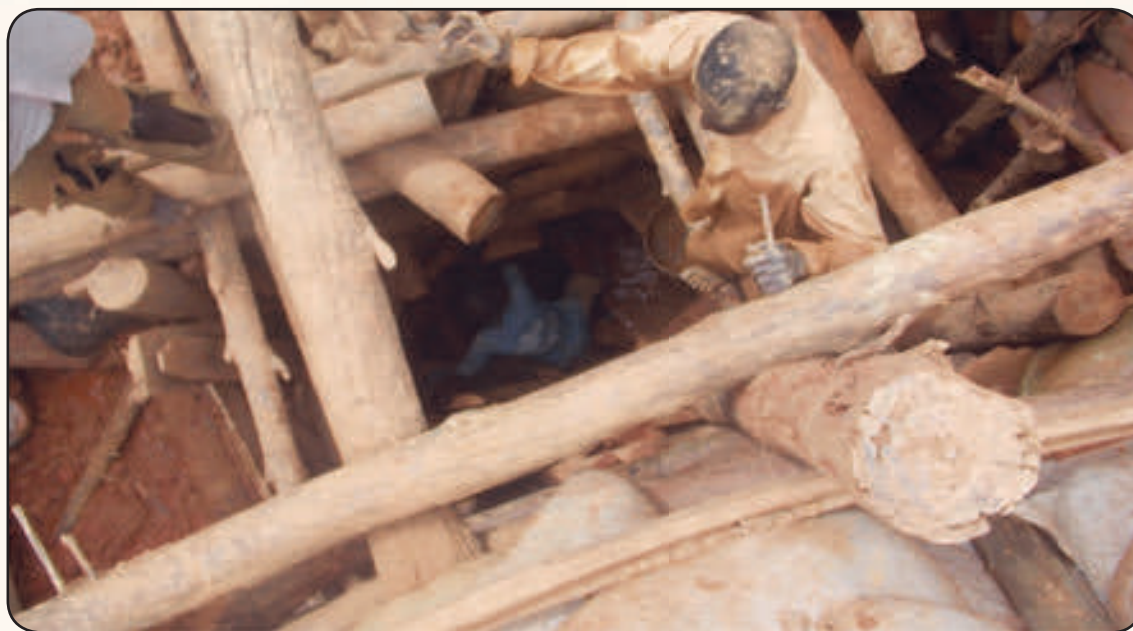
A picture showing a poorly constructed tunnel for gold mining. Photo by Heart Beat Africa Project
