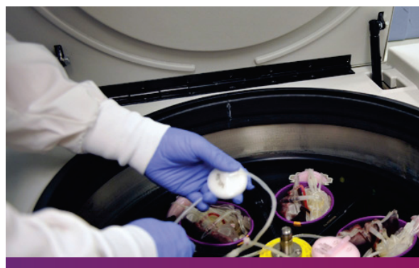
A centrifuge that separates blood into the different components for transfusion. ©AMERICAN RED CROSS SOCIETY
